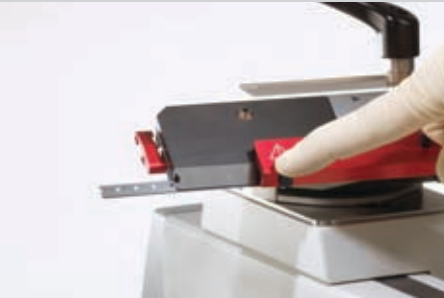
Safer blade removal
