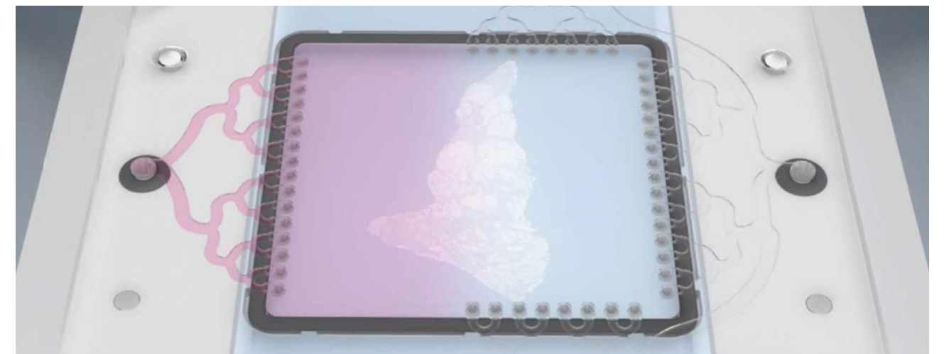
Reagents flow through microfluidic channels, entering and filling the staining chamber.
