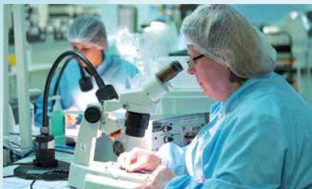
The products are regularly inspected during the manufacturing process. For some products, inspection is carried out on 100% of them.
